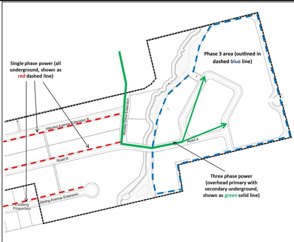
Figure 3 –southern portion of the West End comprehensive development proposal showing conceptual power schematic as proposed by the Developers.
