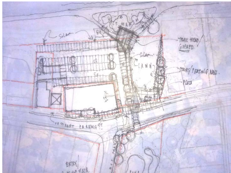
Figure 4-2 - Example of potential increase of public parking at East End Gateway showing an estimated 43 additional parking spaces.
