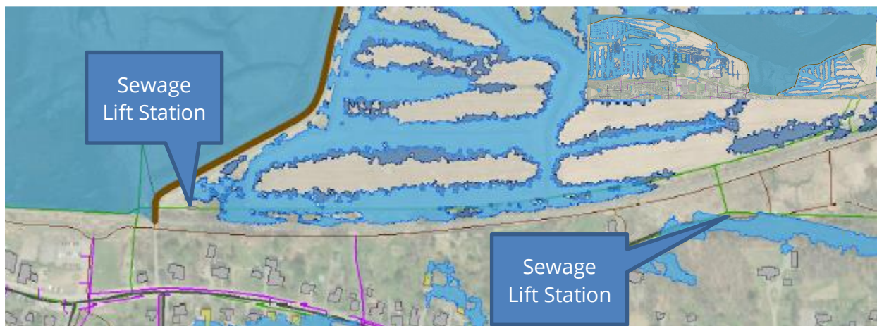
Figure 8.10: Sewage Lift Stations at Risk of Flooding
