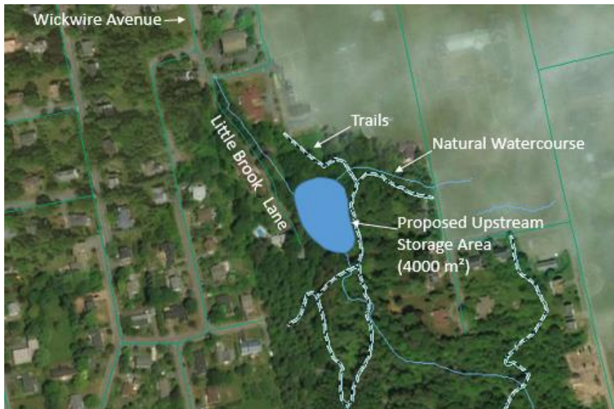
Figure 8.17: Proposed Stormwater Storage Area in open space near top of Willow Avenue
