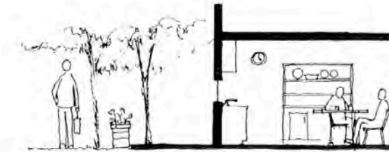
Kitchen entry on public front (window affords privacy)
