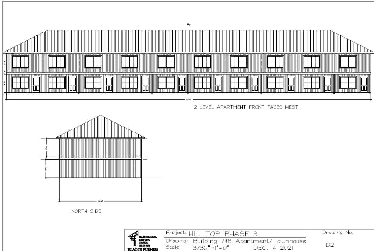
Figure 6 – Front western elevation and north side elevation of buildings #7 & #8, two-storey townhomes.
