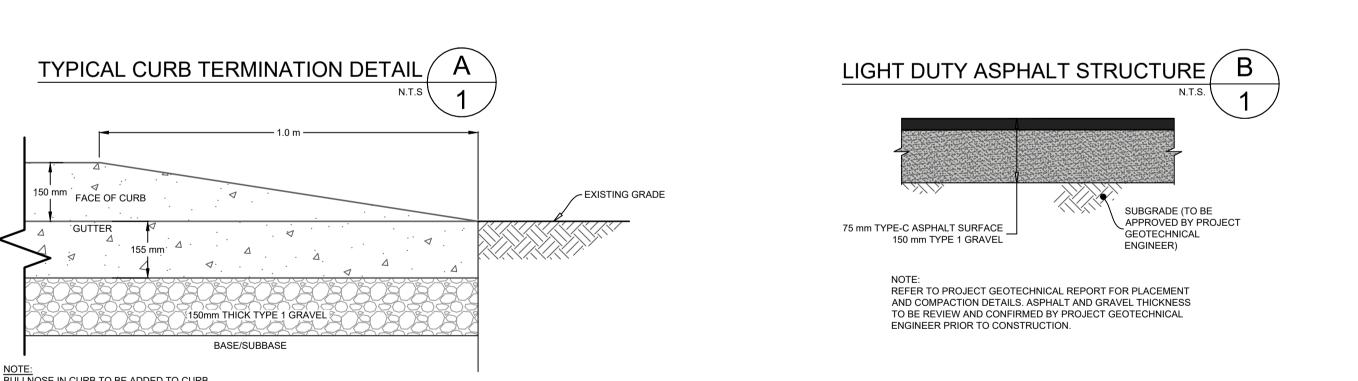
NOTE: BULLNOSE IN CURB TO BE ADDED TO CURB TERMINATIONS WHERE THERE IS NO EX. CURB.
